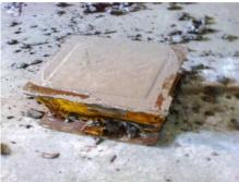
Fig 2: Compressive Strength Cube
